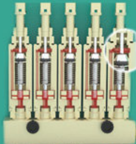
5. The Piston moves and pushes the plunger such that the port on the plug is closed. Injector remains in the position till there is pressure in the main / inlet line.
