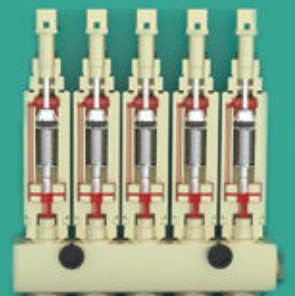
4. The Plunger is pushed down against the spring.
