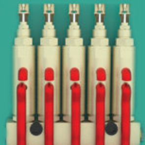
8. In the cycle the grease in discharge chamber is pushed out to the lube point / bearing
