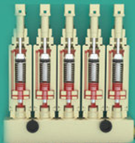
6. As soon as the pressure in the main line drops, the plunger is moved to its original position, opening the part to discharge the chamber.
